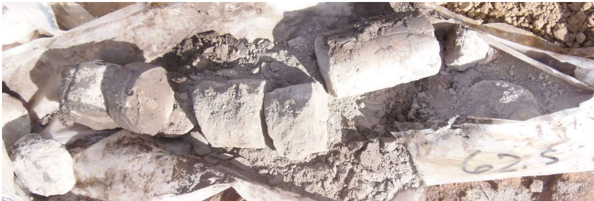
MW-11 59 – 62.5 ft Clay / Shale
