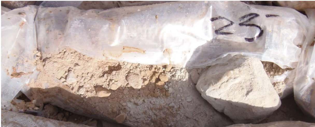
MW-11 20.5 - 23 ft Silty Sand with boulder
