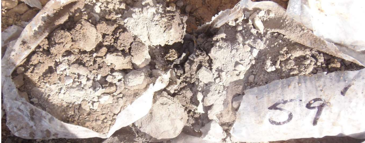
MW-11 57 - 59 ft Clay / Shale
