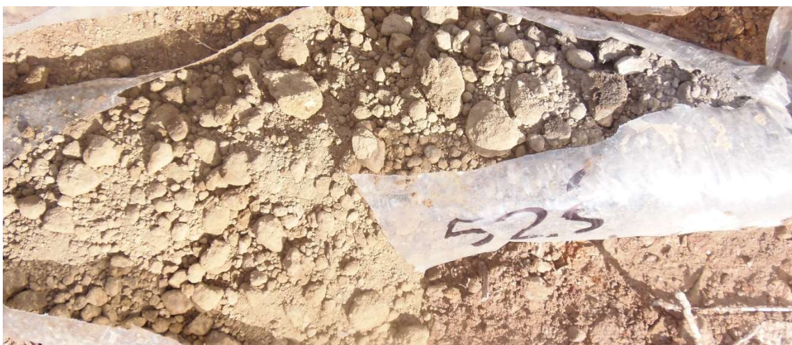
MW-11 50 - 52.5 ft Some clay / shale with some Silty Sand
