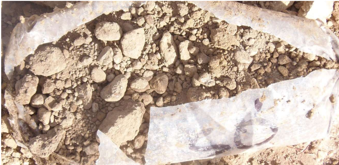
MW-11 49 - 50 ft Some clay / shale with some Silty Sand
