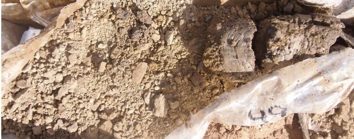
MW-11 47 - 49 ft Silty Sand with intermittent clay/shale
