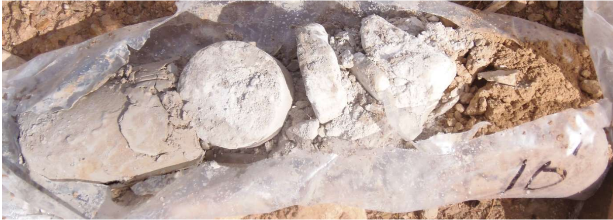
MW-11 7.5 - 10 ft Silty Sand with boulder
