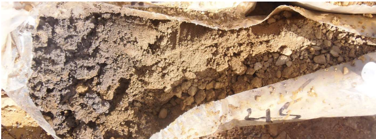
MW-11 43 - 45 ft Silty Sand with intermittent clay
