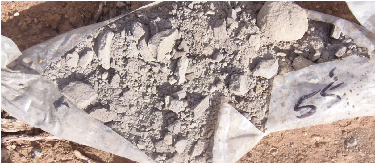
MW-11 52.5 - 55 ft Clay / Shale
