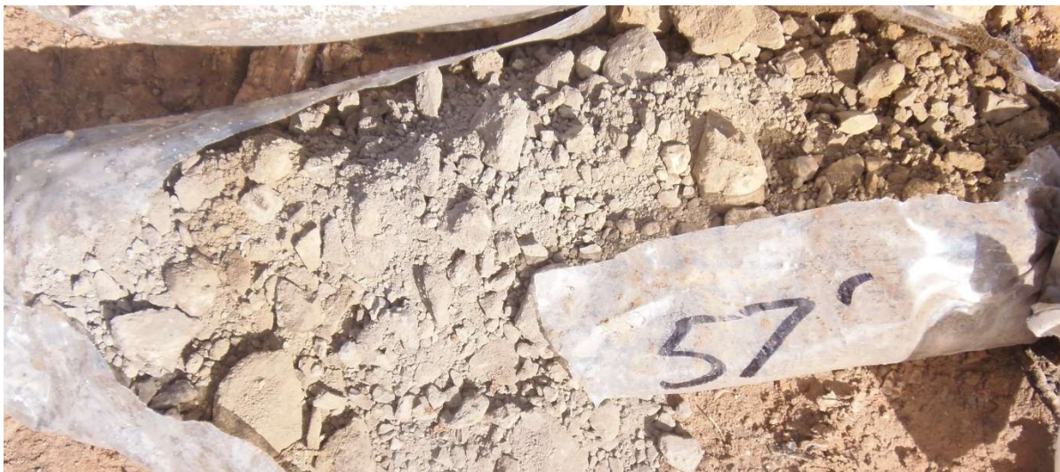
MW-11 55 - 57 ft Clay / Shale
