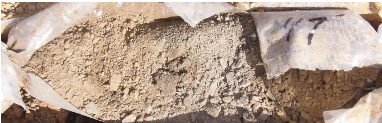
MW-11 45 - 47 ft Silty Sand with intermittent clay/shale
