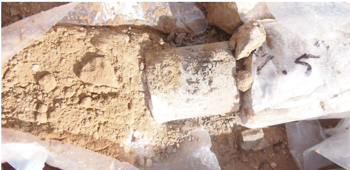
MW-11 5 - 7.5 ft Silty Sand with boulder
